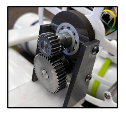
The buoy floats on two PVC pontoons and carries the radio, GPS, and tether reel. The tether retraction mechanism consists of a constant-force spring, gears, and a spool. The 2:1 gear ratio halves the amount of spring travel required to fully extend the cable.
