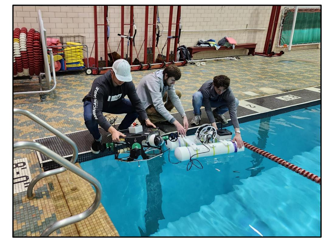
The goal of the RoboSub project (also known as GUAVA) was to create a fully autonomous vehicle for lake exploration and data recording. This data is primarily in the form of video footage of dams and fish habitats that can be used by PA DCNR and the Fish and Boat Commission. This project was a collaborative effort between our senior design team, consisting of both mechanical and electrical engineers, as well as a computer science senior design team.
