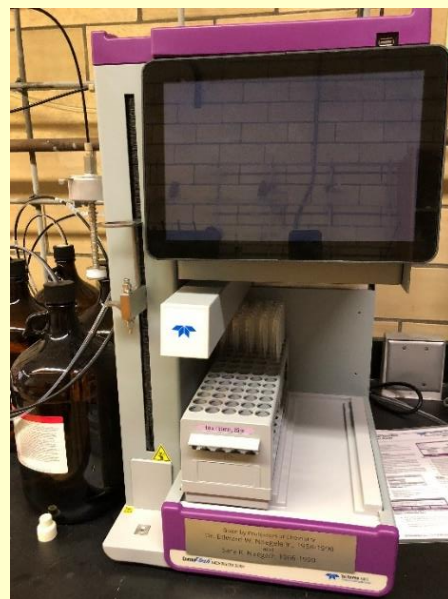
CombiFlash Nextgen 300 instrument is used for chromatographic separation of inorganic and organic mixtures.
