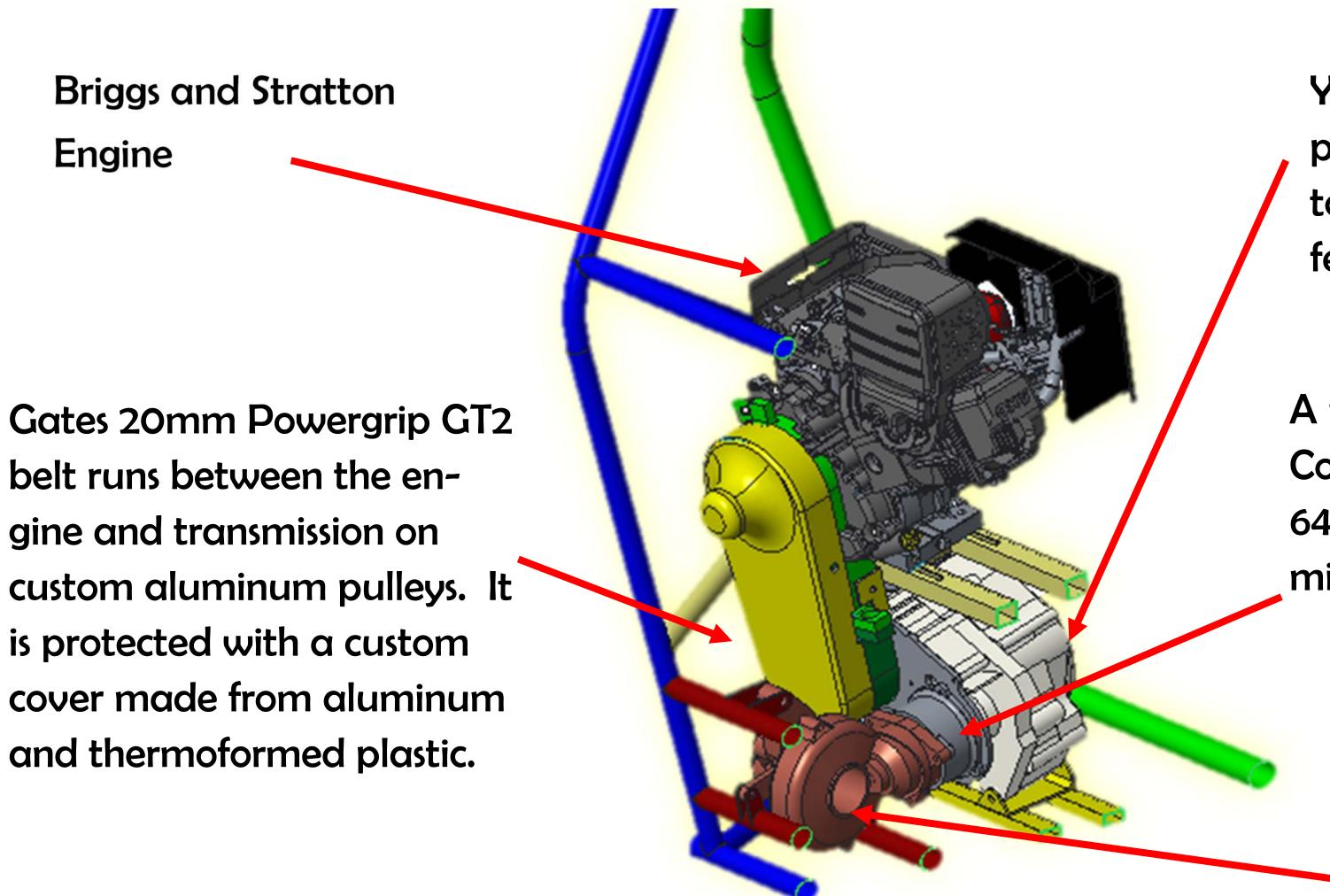
Yamaha XT225 transmission with custom plate cover and collar tightens locational tolerances between transmission and differential.
